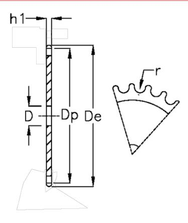
C = 2 D = 14 De = 87.5 Dp = 79.59 For chain size = 3/4 x 7/16 For chain type = 12 B-1 h1 = 11.1 Sumber of teeth = 13
